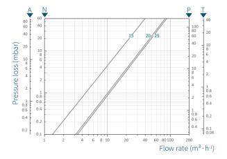
A: air 1.2 kg · m<sup>-3</sup> N: natural gas 0.75 kg·m<sup>3</sup> P: LPG 2.0 kg·m<sup>-3</sup> T: town gas 0.55 kg·m<sup>-3</sup> Gas temperature: 20°C.
