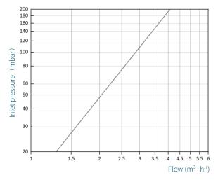
Bypass orifice diameter: 3mm. Air temperature: 20 °C.
