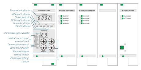
SPC 108 includes a main control module, two 4-channel relay module and a power module. SPC 216 includes two main control module, two 8-channel relay module and a power module.
