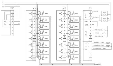
There are four rows of terminals: X1, X2, X3 and X10 on the back of SPC 108. X1 are the terminals for input signal and output signal; X2 are the terminals for output channel  $1\sim4$ ; X3 are the terminals for output channel  $5\sim8$ ; and X10 are the terminals for the input and output of power supply.
