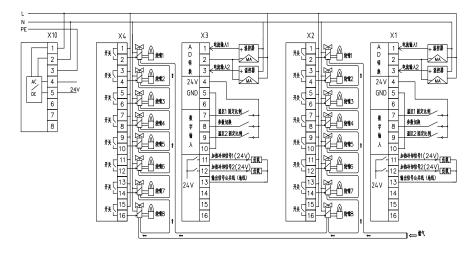
There are four rows of terminals: X1, X2, X3, X4 and X10 on the back of SPC 216. X1 are the first set of terminals for input signal and output signal; X2 are the terminals for output channel  $1 \sim 8$  corresponding to the first set of input signal; X3 are the second set of terminals for input signal and output signal; X4 are the terminals for output channel  $1 \sim 8$  corresponding to the second set of input signal; and X10 are the terminals for the input and output of power supply.
